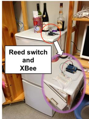
**Figure 4:** Refrigerator hardware. Xbee and reed switch.
