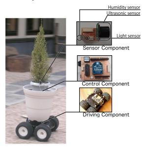
Figure 3. The PotPet prototype.
