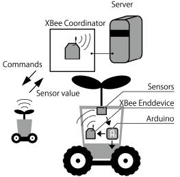
Figure 4. The system architecture of the PotPet.
