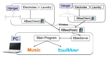
Fig. 3. System architecture of the AwareHanger
