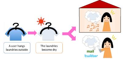
**Fig. 1.** The AwareHanger concept. When the laundry becomes dry, this system helps a user bring it in efficiently by informing him/her of its readiness via several media: by sound when at home or by Twitter when out.
