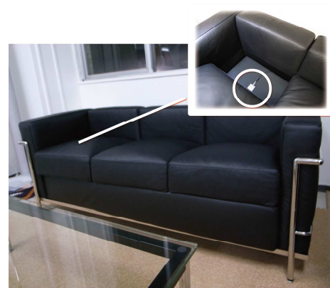
Figure 4. Sensor placement in sofa.
