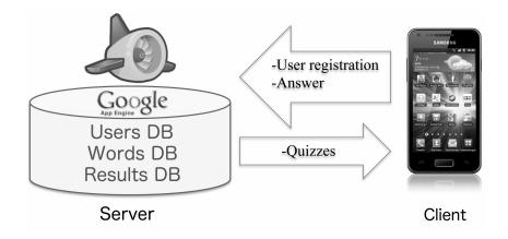
Fig. 3. Server and client configuration
