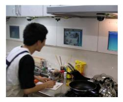
**Fig. 4.** A user is cooking while replaying the recorded pictures and sounds of the cooking process on the LCDs. The images are displayed on one of the four LCDs at the workplace. When he completes the displayed step, he can view the next step by pressing the foot switch.
