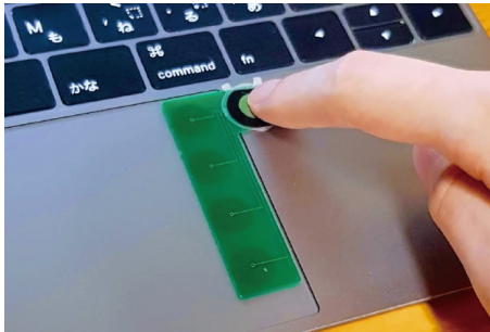
Figure 1: Ohmic-Sticker with 2.5 DoF comb electrodes pattern; Ohmic-Sticker works simply by attaching to a commercial touch surface.
