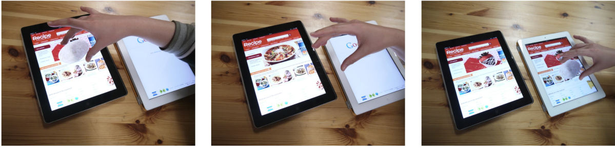
Figure 1: Proposed drag-and-drop method between two computing devices. A user picks up a data object (left) from one device using their fingers, (center) brings it to another device, and (right) puts it down on that device.
