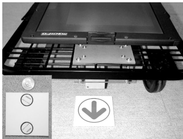
Figure 3: Position and direction of the cart are calibrated by reading the marker plate (center) inlaid with two RFID tags on the underside (left).
