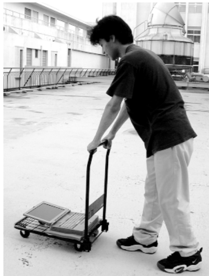
Figure 1: The Virtual Glassboat system. The cart mounted display scrolls with the movement of the cart to provide the illusion that the user is looking underground.
