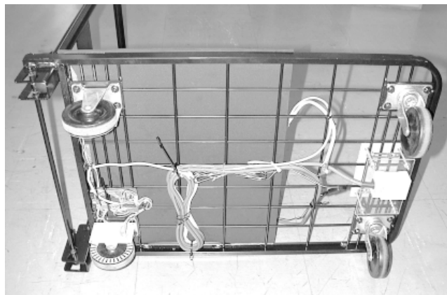
Figure 2: Underside view of the Virtual Glassboat. Optical sensors detect rotation of the rear wheels (left). The RFID reader
