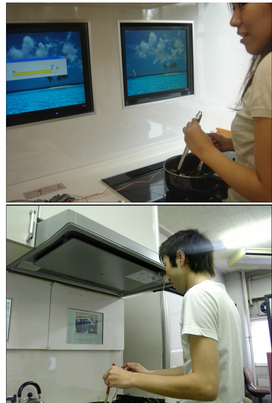
Fig. 5 Actual example of the display. Live view and salinity bar-graph.
