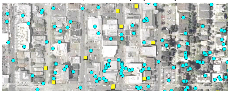
Fig. 2. An overhead satellite map showing the results of self-mapping using the hotspot finder seed set. The squares mark the locations of the beacons in the seed set, while the circles denote the beacons placed by the self-mapping algorithm
